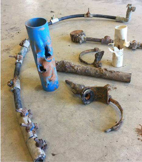
**Burst water mains, a 6-foot service line with multiple repairs, and rusting, corroded pipes and valves illustrate the need for addressing aging water infrastructure in the county.**
